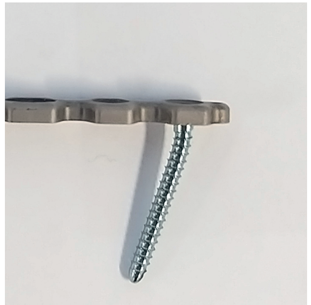
Locking Screw Angle Stability Results
