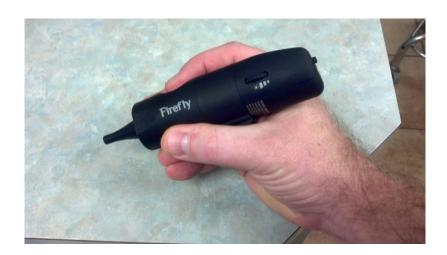
On the side is a dial that controls the brightness of the light. Most of the time I left it at the brightest setting, though this may vary based on your individual preferences.
